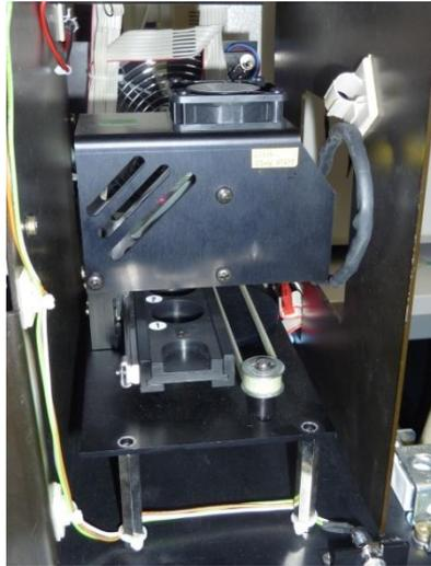
The whole module is fixed with only 4 screws (2 at the front, 2 at the rear). These screws can be opened using a 4mm Allen key. Before removing the module the 2 red CAN connectors, one below the halogen board and the other at the filter slider motor), as well as the blue connector from the optical sensor must be removed.
