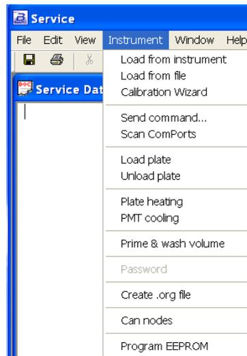
This mode requires the use of specifically modified Berthold Technologies drivers. Otherwise the device driver cannot be installed successfully because of a different vendor ID of the USB device. Run the service software and scan the com port to identify the NightOWL (with not programmed EEPROM). If found select the NightOWL entry in the found instruments list and select "Program EEPROM" from the "Instrument" menu.
