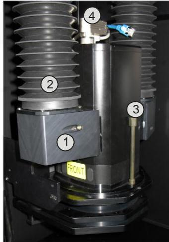
Fix the camera with the 2 fastening screws (3). The power supply (4) is connected through a 7 pin Tuchel connector. This connector is on the camera face plate and connects to the power supply connector on the camera plate.
