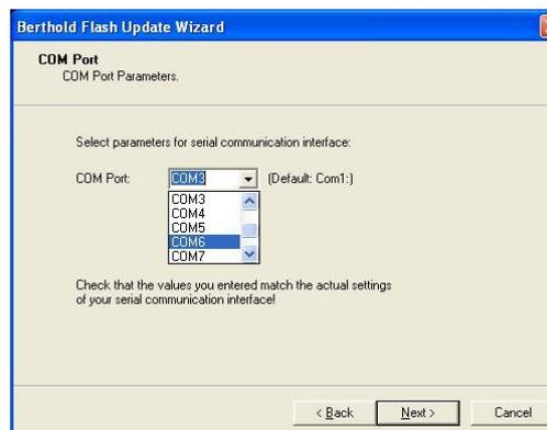
In this Dialog box you have to select the Com port, where the NightOWL is connected to. Although we are using the USB or Ethernet to communicate with the NightOWL there is always a virtual Com port installed in the system. Check your Windows device manager to find out the correct COM port.
